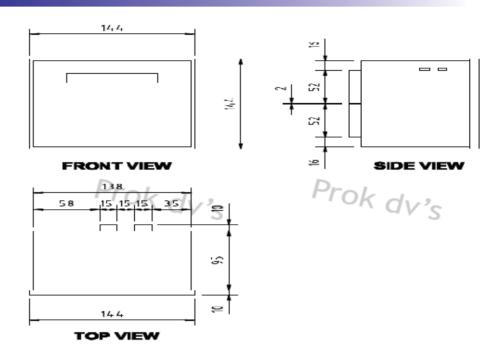
NOTE: ALL DIMENSIONS ARE IN MM TOLERANCE:- ± 1MM
